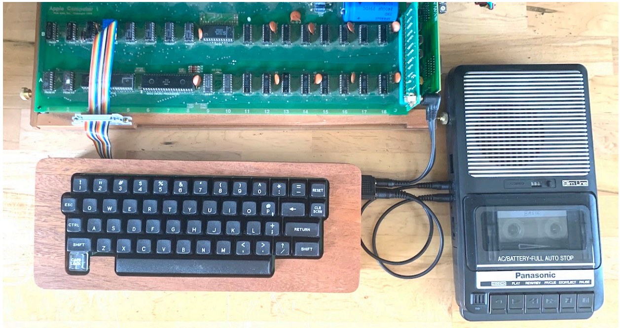
Figure 7 Keyboard Tape Player Connection
